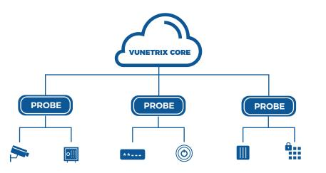
The complete Vunetrix Network Monitor (VNM) solution includes patented Core hardware and Probe software. The Probe software pings devices to collect health and performance data and communicates security with the Core – which processes device metrics and alerts, stores data, and authenticates/controls users and groups. All of this system health and status information is made visible and actionable via the Vunetrix SMART Dashboard.
