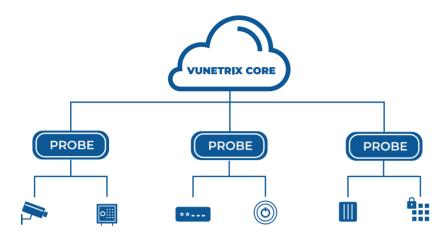
The complete Vunetrix Network Monitor (VNM) solution includes patented Core hardware and Probe software. The Probe software pings devices and applications to collect performance data and communicates securely with the Core – which processes device metrics and alerts, stores data, and authenticates/controls users and groups. System performance and status information is made visible and actionable via the Vunetrix SMART Dashboard.
